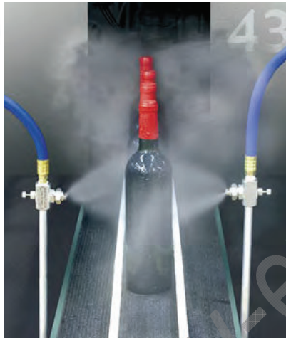
(2) Model EB1040SS nozzles are used to rinse wine bottles after capping.
