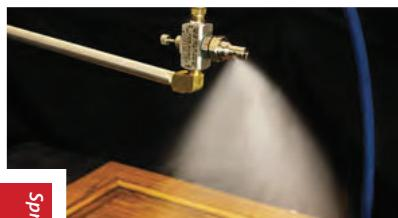
A Model AD1010SS is used to apply a protective coating to wood panels.
